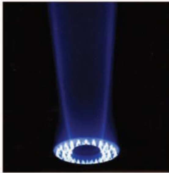
Figure.I.1: Photograph of the so-called Sandia D flame. The central jet (25% methane and 75% air in volume) is surrounded by 72 pilot flames (mixture of C 2 H 2 , H 2 , air, CO 2 and N 2 ) [5]
