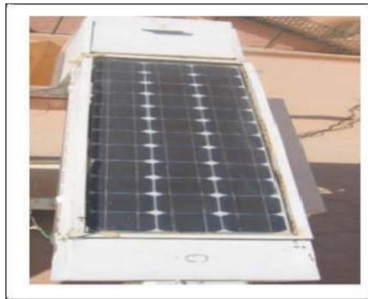
Figure I-4: Image of the hybrid collector studied by TOUAFEK [13]
