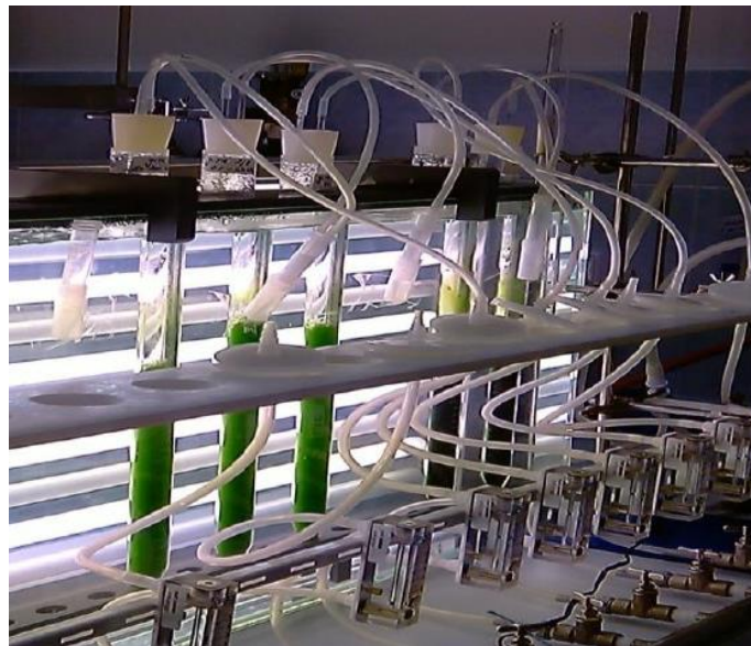
Figure III.1: Batch cultivation of C. vulgaris in lab-scale photobioreactor (Ghobrini, 2022).
