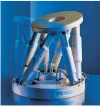
Figure 3.8 Le robot Roboscope
