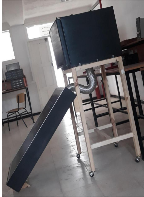
Figure III.9 Box Linked to Drying Chamber via Aluminum Duct; Fans Wired in Parallel with Cut-off Switches.
