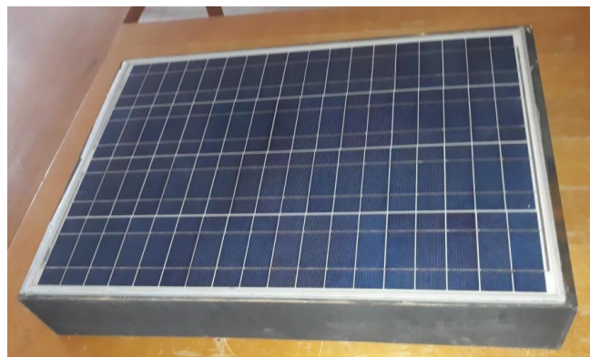
Figure III.6 Installation of the Solar Panel on Top of the Box.
