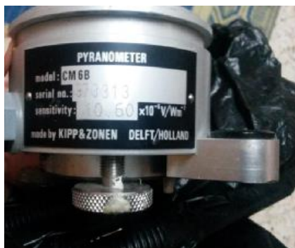
Figure III.36: Pyranometer for illuminance measurement.
