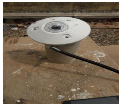
Figure III.36: Pyranometer for illuminance measurement.
