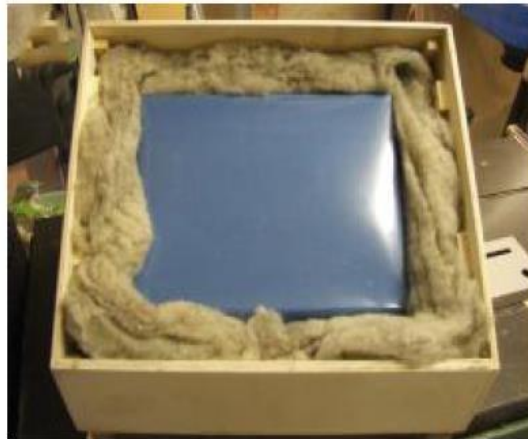
Figure III.19: Assembly of the Box and Basin [11].
