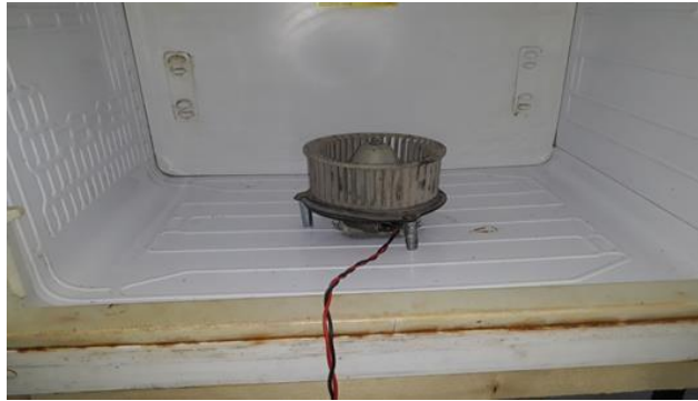
Figure III.7 Fan Installation for Preventing Food Spoilage During Drying.
