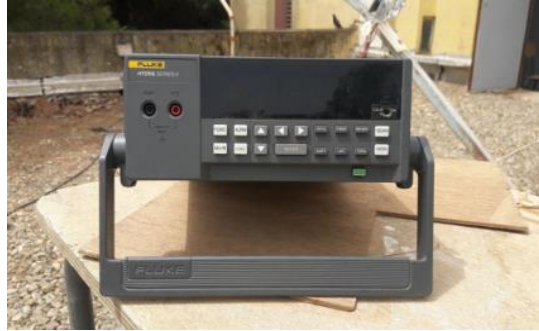
Figure III.35: Data logger type FLUKE HYDRA SERIES II.
