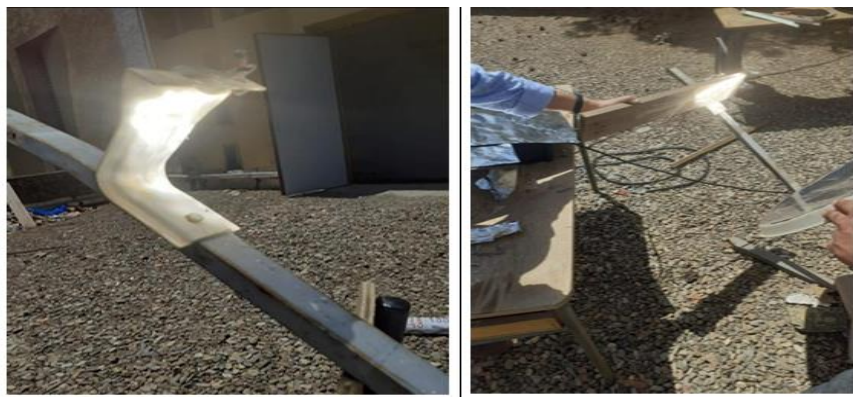
Figure III.32: Determination of the focus of the dish
