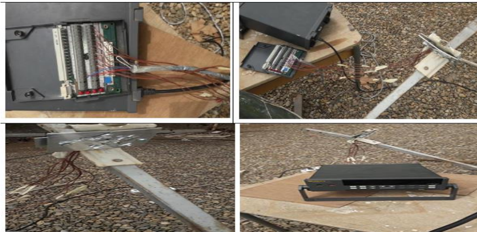
Figure III.34: The location of thermocouples in data acquisition
