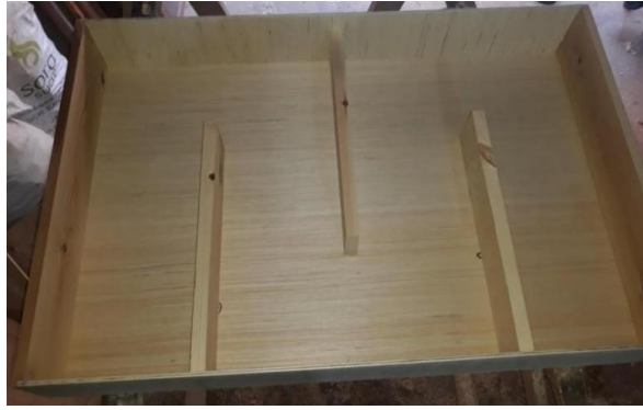
Figure III.1 Formation of a Serpentine Air Channel Using Wooden Boards.
