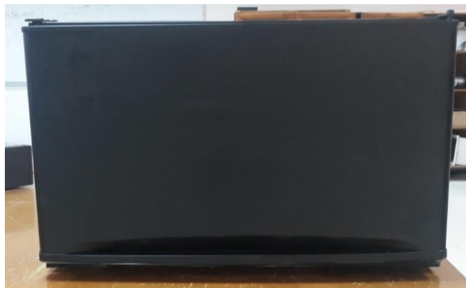
Figure III.8 Black Coating of Freezer to Prevent Light and Preserve Food Composition.
