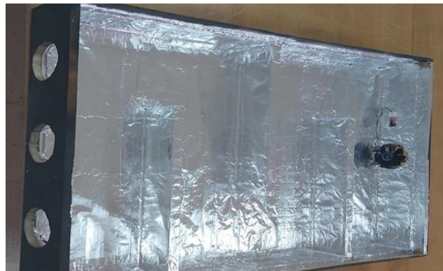
Figure III.5 Computer Fan Installed to Draw Hot Air into Drying Chamber.
