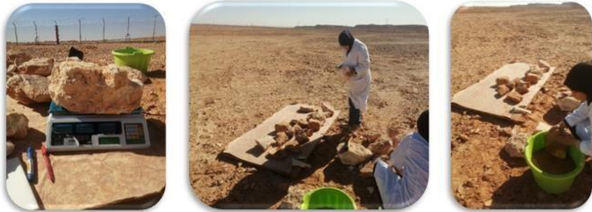
Figure III.9. Collected and stones preparation :: Cleaning;Drying andWeighing
