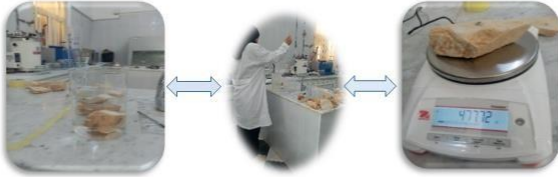
Figure III.15. Density measurement stages
