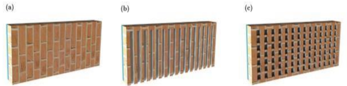
Figure II.9. Illustration of the different internal surface structures of the north wall [20]
