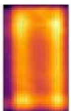
multiple activated by-pass diodes affecting 2 over 3 of module
