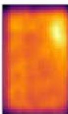
warning hot spot on a thin-film module
