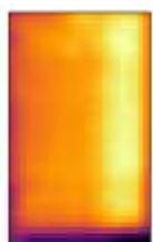
warning activated by-pass diode typically 1 over 3 of the module
