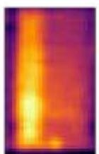
activated by-pass diode typically 1 over 3 of the module
