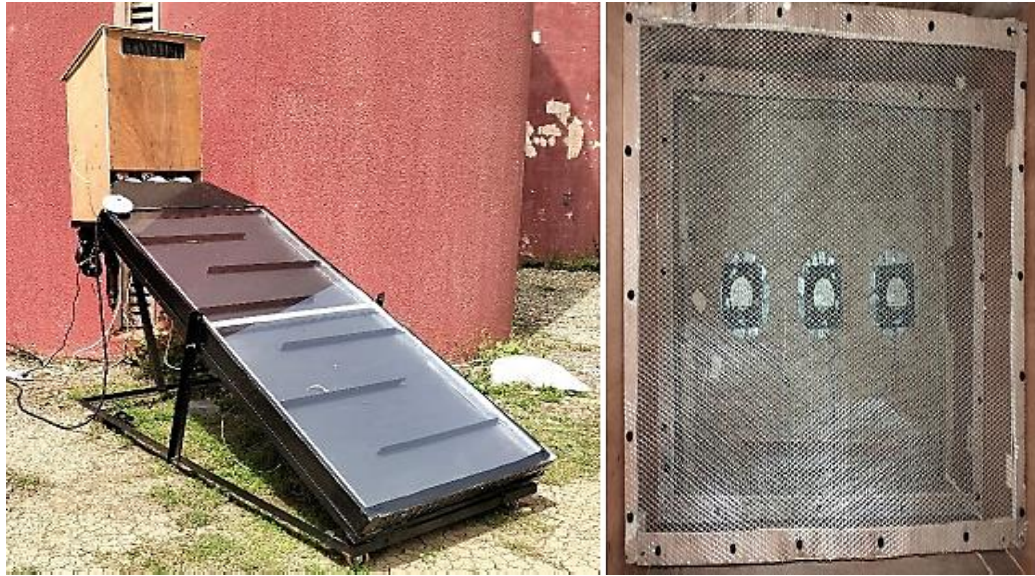
Figure I.27: Active or forced indirect solar dryer and drying chamber [2]
