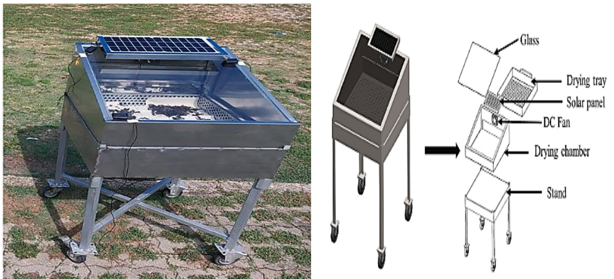
Figure I.22: photo and Graphical representation of solar dryer [27]
