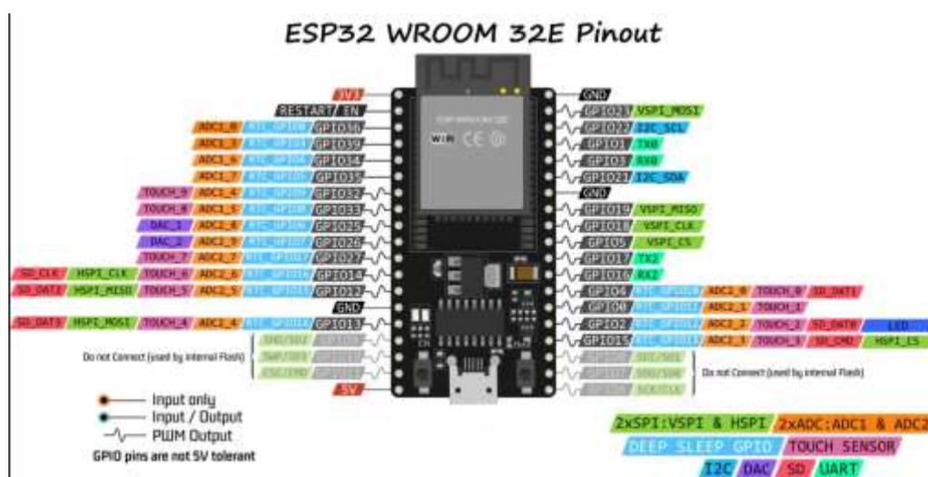
FIGURE 4.1 – ESP32 WROOM 32E PINOUT
