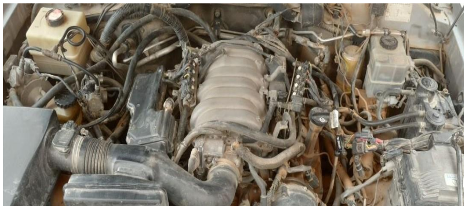
Figure 3-14: Assemblage final du kit GPL.
