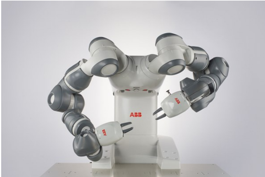
Figure 1.5: YuMi .Abb’s Dual -arm robot [11]
