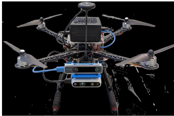
Figure 1.18: UAV frame with mounted drivers, companion computer and payload [31].
