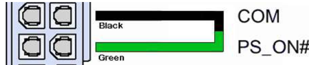
Figure 3.14: Power-on of the ATX-450W power supply
