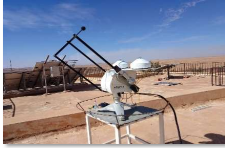
Figure 3-13: SOLYS 2 solar radiation tracking and measurement system at URAER
