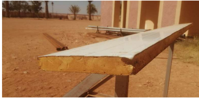
Figure 3-9: Sandwich panel material used in the experimental building
