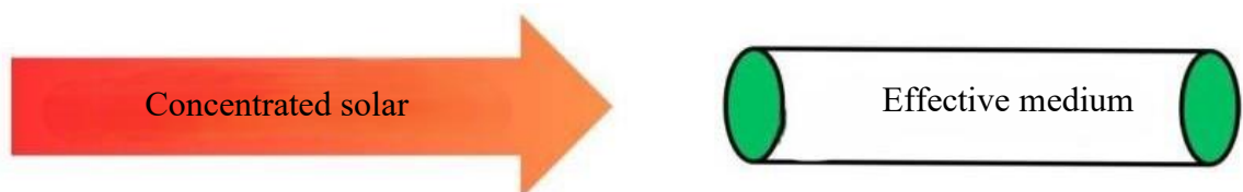
Figure (2-27): End-pumping method.
