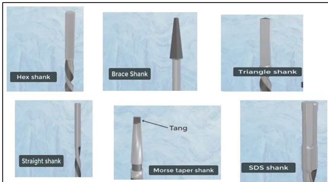
Figure 29. Classification of drill bits depending to the shape of shank
