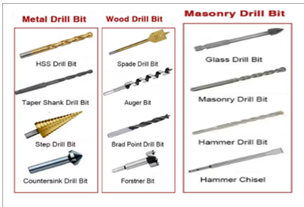
Figure 30. Drill bit depending work piece
