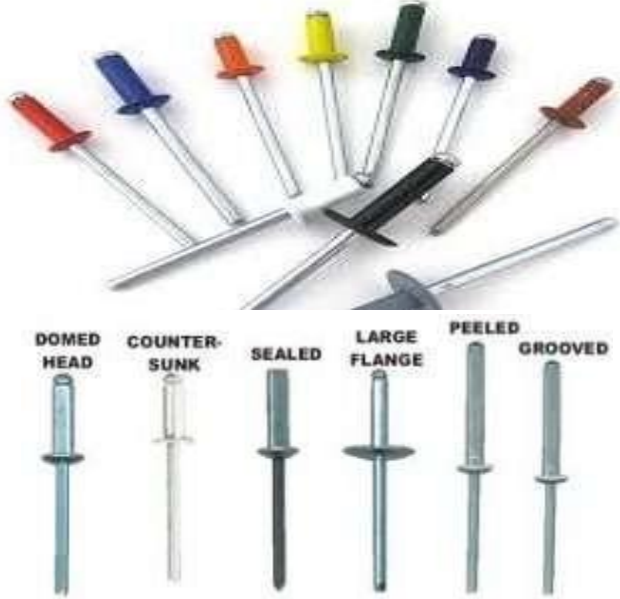
Figure 43. Blind rivets types
