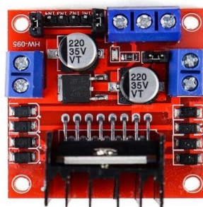
Figure (III – 15): L298N motor driver.
