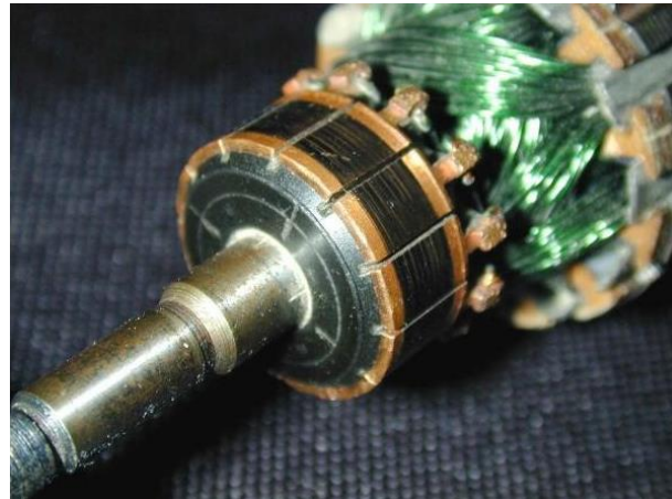
Figure (I – 4): collector of DC motor
