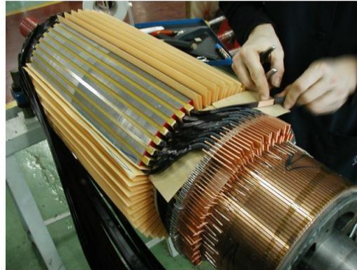
Figure (I – 2): the armature of DC motor (rotor)
