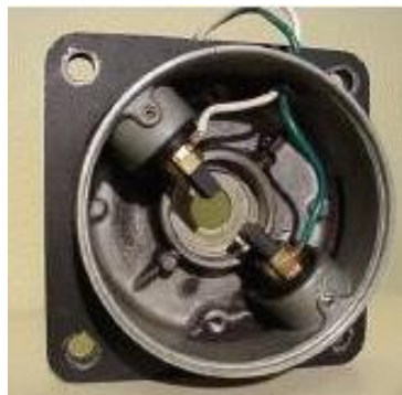
Figure (I – 5): brushes of DC motor.
