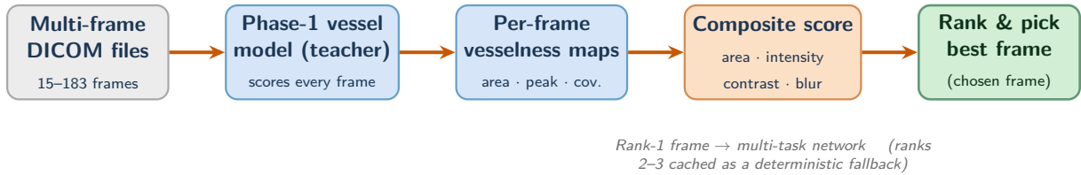
Figure 3.20: The automatic best-frame selection pipeline. Multi-frame DICOM files are decoded; the Phase 1 vessel segmentation model, re-used as a teacher, scores every sampled frame by its vesselness response; per-frame vesselness maps yield a composite score combining vessel area, intensity, contrast and a blur penalty; and the frames are ranked so that the rank-1 frame is forwarded to GCT-Net, with ranks 2–3 cached as a deterministic fallback.
