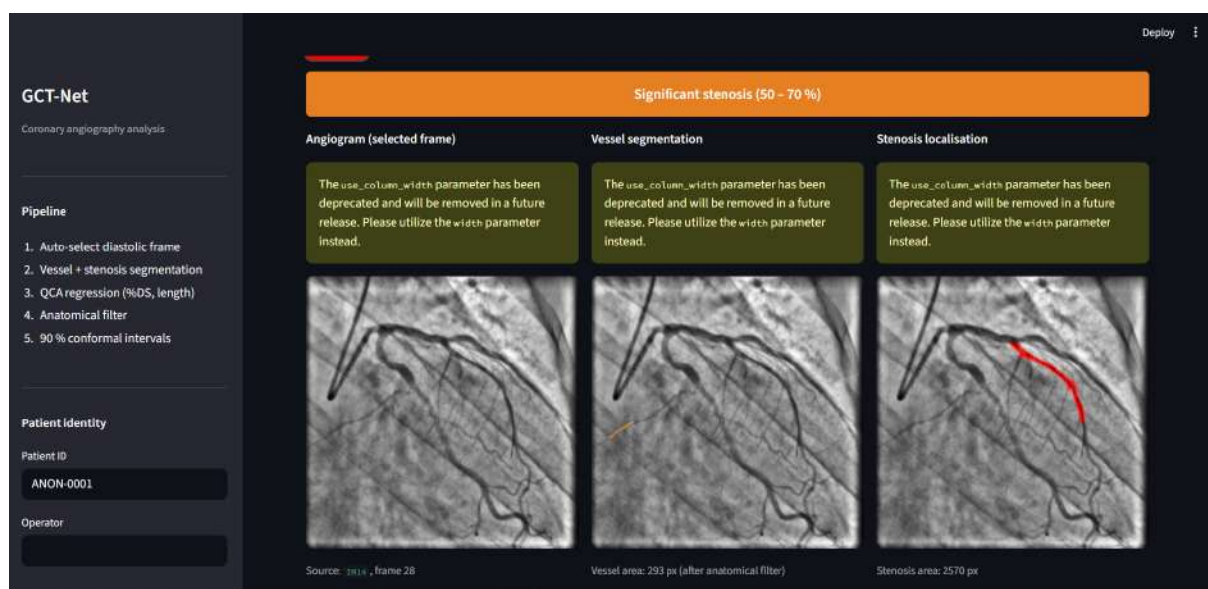
Figure 3.47: Web application — segmentation outputs. After analysis, the interface shows the automatically selected angiogram frame (left), the vessel segmentation after the anatomical filter (centre), and the stenosis localisation (right, in red), together with a colour-coded banner classifying the lesion severity (here, a significant stenosis of 50–70%). The vessel and stenosis areas in pixels are reported beneath each panel.
