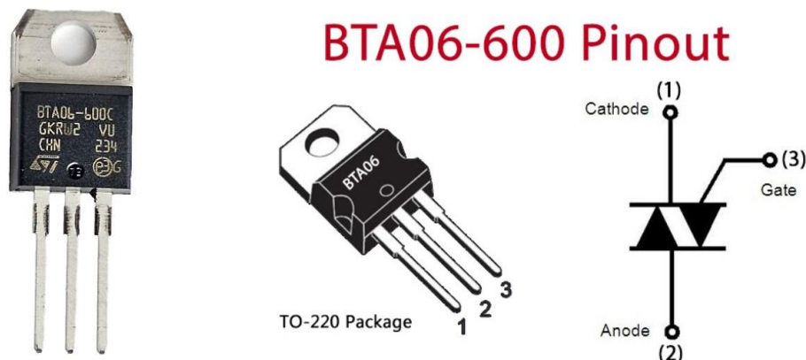
Figure 3.12: BTA06 Triac Picture and Pinout.
