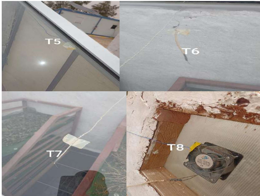
Figure II. 8. Instrumentation of the solar dryers
