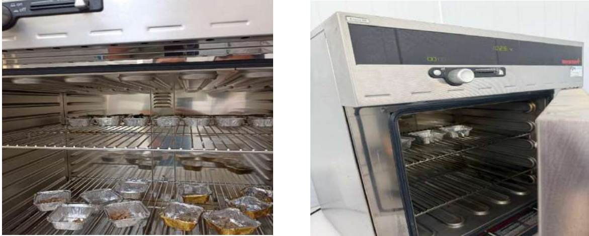
Figure II.12. Photographs of the oven used to determine the dry matter content
