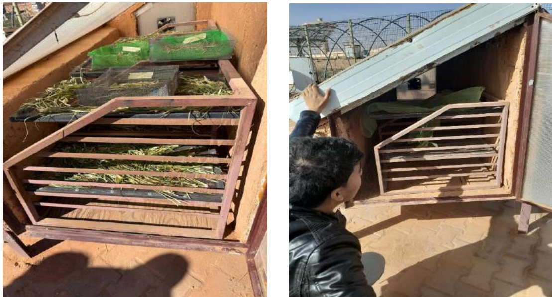
Figure II. 5. Photograph of the drying chamber: Left) Direct solar dryer; Right) Indirect solar dryer
