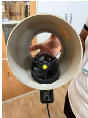
Figure. II.10.1 Anemometer used to measure mass flow rate
