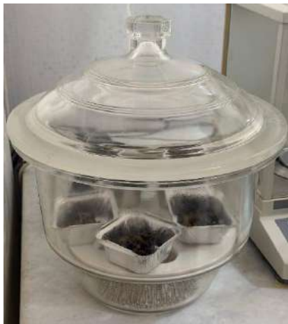
Figure II.11. Photographs of the desiccator used in the process to determine the initial water content.
