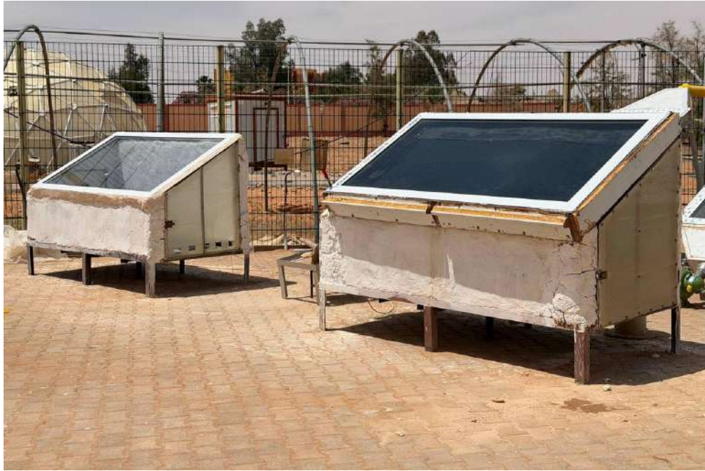
figure.II.14. final look of both dryers after all the renovation labor
