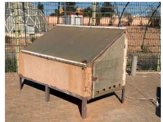
Figure II. 3. Prototype of an indirect solar dryer (before)
