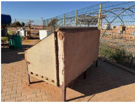
Figure II. 3. Prototype of an indirect solar dryer (before)
