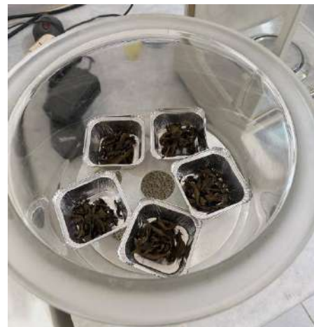
Figure II.11. Photographs of the desiccator used in the process to determine the initial water content.
