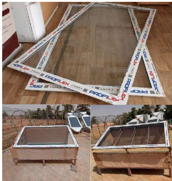
figure.II.12. results of installing aluminum framed 5mm glass panes
