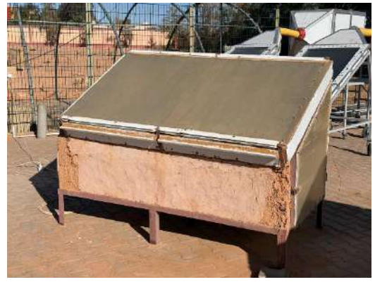
Figure II. 3. Prototype of an indirect solar dryer (before)
