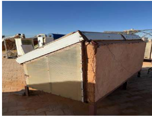
Figure II. 3. Prototype of an indirect solar dryer (before)
