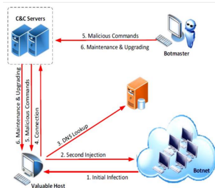
Figure 1.15: Botnet life cycle(28)
