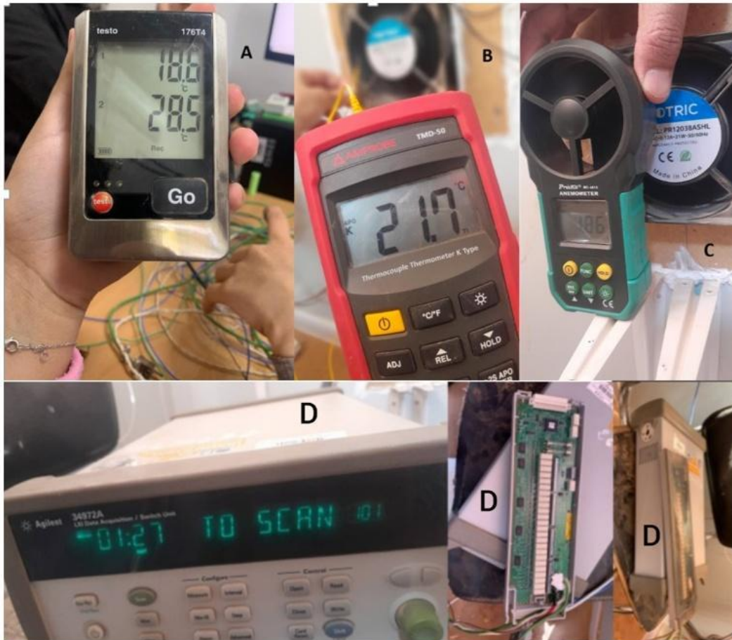
Figure 3-7: Different measuring instruments, A: Testo 176T4, B: K-type thermocouples, and C: Anemometer, D: Agilent 34970a.
