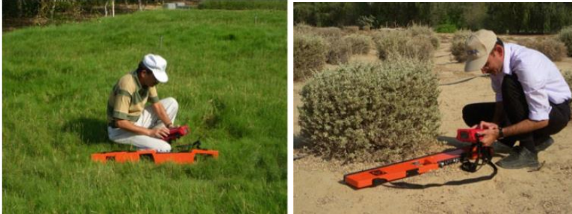
Figure 1. Le Geonics EM38 : (a) mode vertical, (b) mode horizontal.
