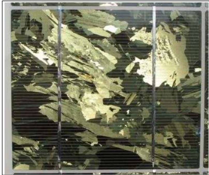
Figure 22 : Silicium poly cristallin
