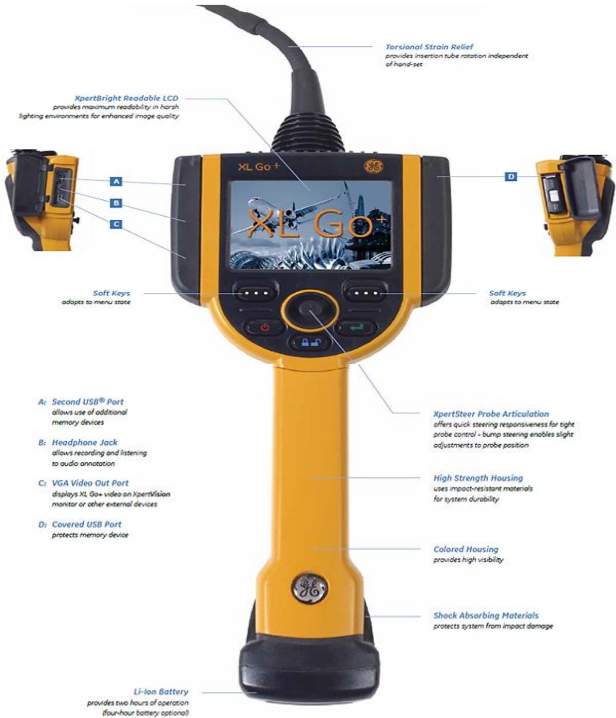
Figure V.2: Different parts of the Borescope XL Go+™ VideoProbe [42].
