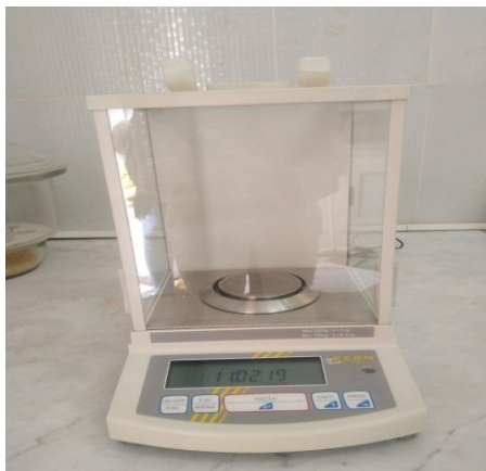
Fig.III.21. Balance KERNABT 220-4M: 20g/0,1m
