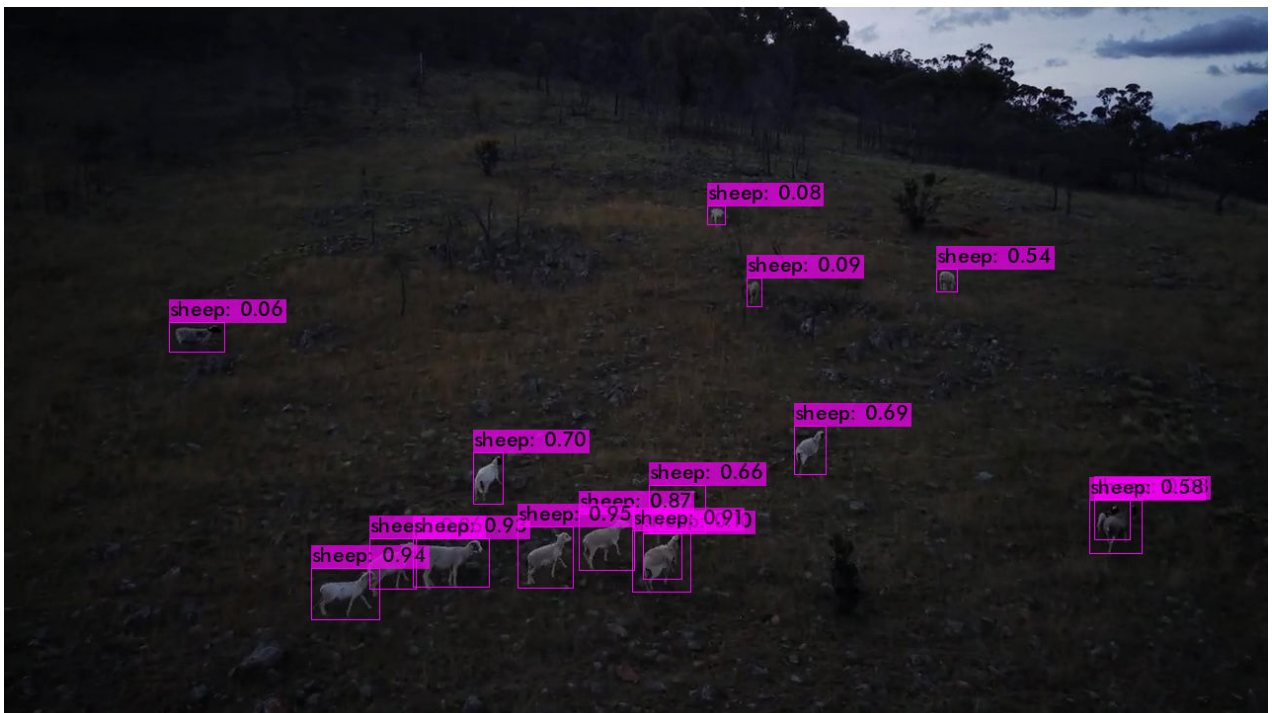
FIGURE 3.9 – Test example of sheep detection from a side view angle in low light
