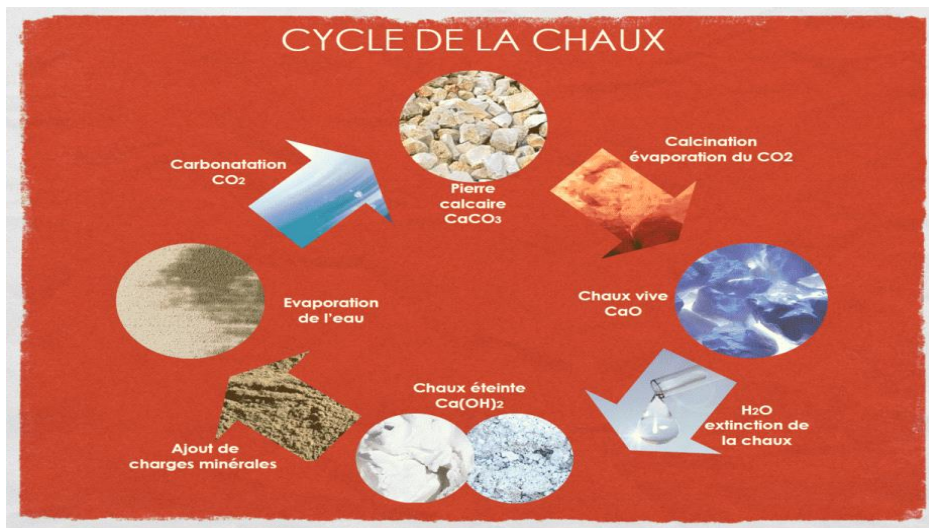
Figure 52 : cycle de la chaux [30]
