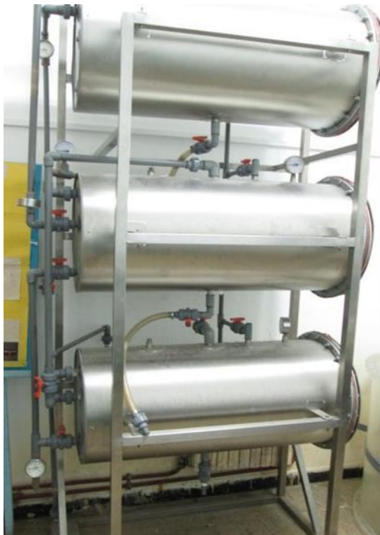
Figure I-29: ENIT-Tunisia URME multi-effects distiller
