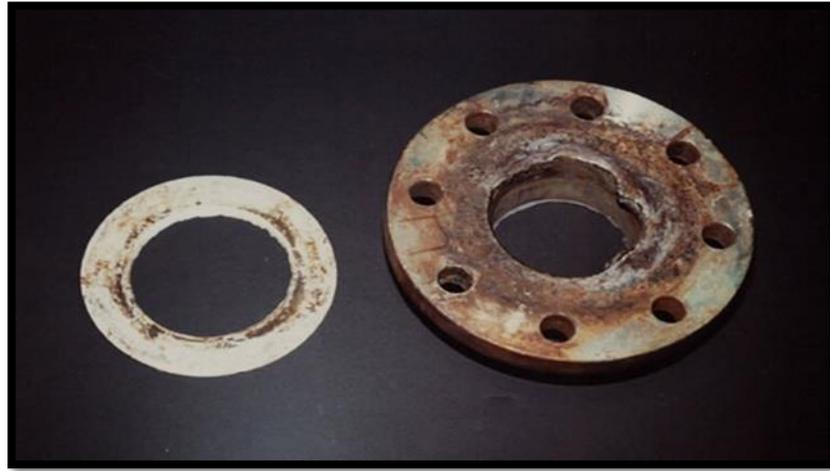
**Figure07:** corrosion cavernouse [8].
