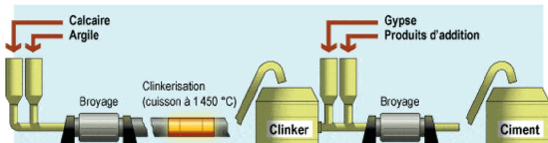
Figure II. 1: Fabrication de ciment
