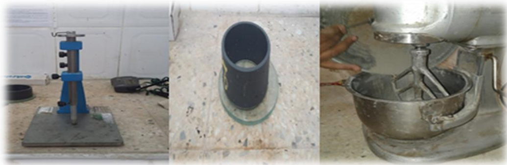
Figure III- 2. Essai de la consistance
