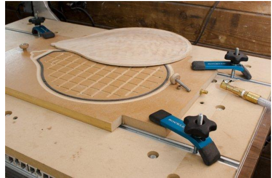
Figure 1-4:T Track Grid Work and Vacuum hold-down method
