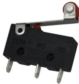
Figure 1-7 : Micro-switch used for limits and homing.
