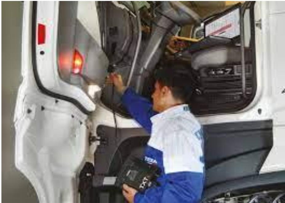
**Figure I:5.Scanner (diagnostic) [13]**
