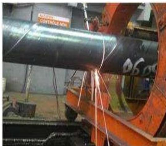
**Figure I.14 :** Processus Oxycoupage de tub
