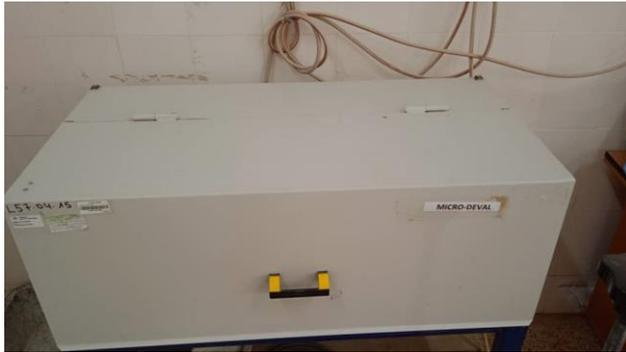
Figure 28: machine Micro D'eval
