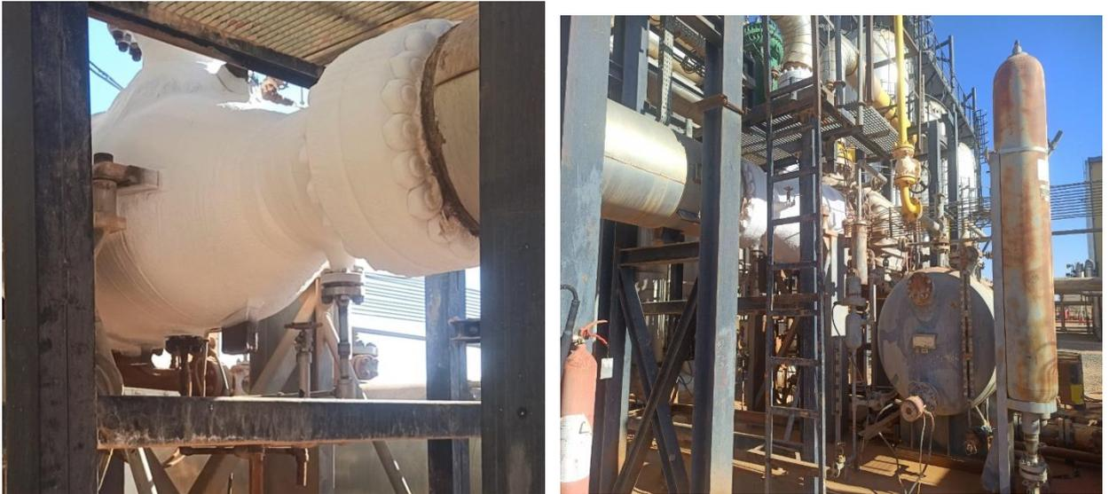
Figure III- 8:le turbo expander [photo réelle]
