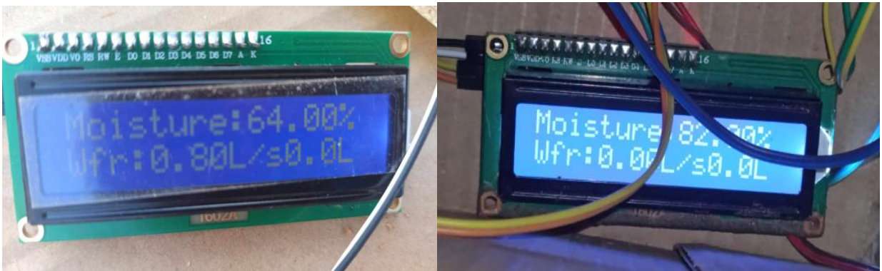
Fig. III. 27. LCD screens for displaying moisture and flow values.
