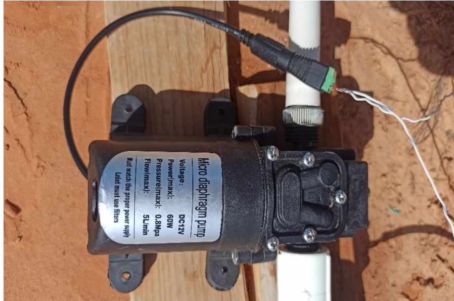
Fig. III. 9. Dc Water pump.
