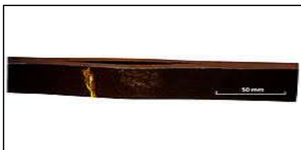
Figure 11:corrosion fatigue [J]
