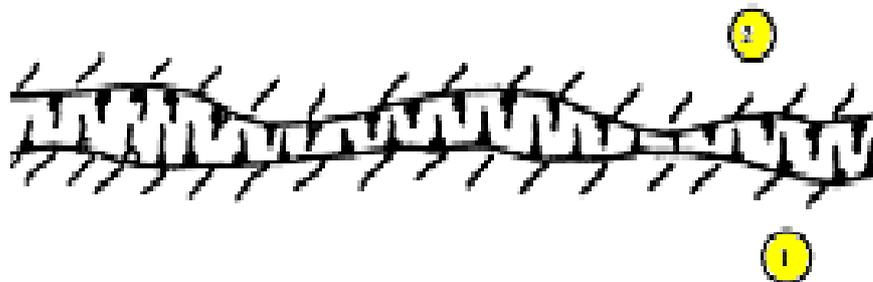
Figure I.12 La lubrification limite[6]
